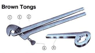
A brown tong is used for holding or lowering short strings of rod or casing. By turning a wing bolt it can be adjusted to accommodate all sizes from RW drill rod to AW casing.
