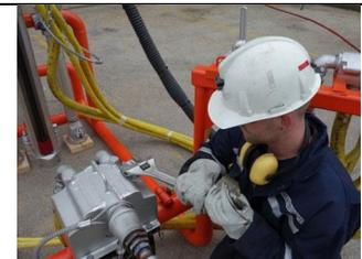
Everything is now ready for the operator to begin drilling. The operator should conduct a safety routine of checking all nuts that should be tight to hold the drill in place before opening the air to the remote control panel. If a crucial nut is missed and is not tight the heavy drill assembly could fall and injure the driller.
