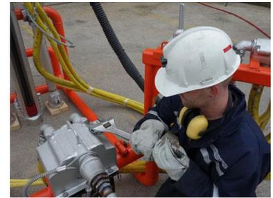
The operator needs only look into the lubricator to determine if there is lubricant or if it is empty. The lubricator is simple to fill with a proper spouted container. Be sure to keep rock drill oil clean before using.
