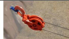
The hook on the end of the 5/8 inch cable is fixed to a metal loop provided on the lower cross bar of the upright drill mounting tubes of the drill sled.
