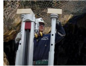
Once the two column bars have been extended with proper blocking in place with the two column bars well aligned at right angles to the back and above and the floor below the operator must tighten the ratchet jacks at the bottom of the column bars to make the entire setup rigid and strong.
