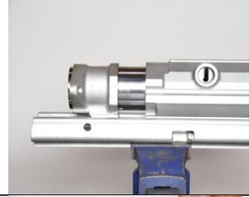
79. Examine the bronze Front Cylinder Liner (30) in the Front Cylinder (31) for signs of scoring or wear. The liner ensures good compression in the rock drill and should be replaced at the first sign of scoring or wear.
