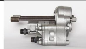
102. Remove the two loose Studs (37) and two Nuts (36) and two Lock Washers (37) used to hold the SASTANMO to the Feed Shell. Examine the studs and nuts and washers for wear or damage and replace if necessary.
