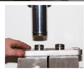
125. Use the fifty ton hydraulic press (on low pressure) to push out the one Bearing (27) from the Front Cover (8).
