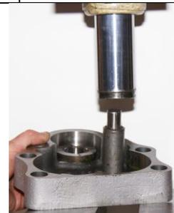
126. Use the fifty ton hydraulic press (on low pressure) to push a new Bearing (27) into the Front Cover (8).
