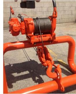
The side view picture at the left shows the brake lever in the fully open position. One can see the cable from the overside of the drum of the AW80 hoist going to the first pulley block connected by a hook to the lower cross bar of the drill mount portion of the drill sled. The cable exits to the right towards the second pulley. One can see the return cable hooked to a lower metal loop provided on the cross bar.
