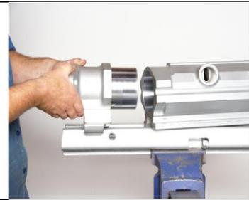
78. To install the Front Cylinder Washer (31) into the Cylinder (43) the two parts should be slid into a short length of guide shell (from the Feed Assembly) and tapped with the rubber hammer to set the two parts together with correct alignment of the ways of the two parts before the Front Cylinder Washer is press fitted into the Cylinder (43) using the fifty ton hydraulic press in the shop
