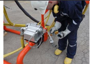
After examining the lubricator filter and checking the oil is sure that the filler cap is securely tightened with a mine wrench.
