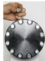
212. Insert the two Studs (17) four Copper Washers (15) two Banjo Fittings (16) and two Nylock Nuts (14) into the two air inlet holes in the head of the Support (18) to complete the air fittings
