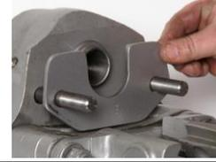
150. Place the two Nuts (3) on the ends of the Bolts (14). Slide the large Square Head Bolt (11) through the holes in the Left Motor Clamp Support (12) and Right Motor Clamp Support (28) and thread on the Nut (30).
