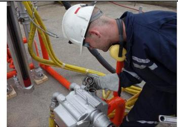
Remove the air hose feeding the lubricator and one can access the filter that is installed in the lubricator. The stainless steel filter should be examined for excess debris and blown clean with an air hose before re-installing. Always “blow” the main bull hose before connecting to the lubricator to ensure any debris from the mine pipe system or accumulated water does not enter the lubricator.
