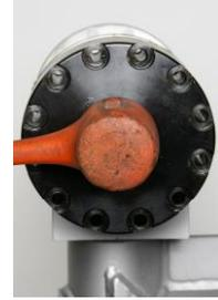
211. Install the twenty-four Cap Screws (1) and twenty-four Nuts (10) through the Cylinder (2) and head of the Support (18) (Twelve per side). Tighten with the impact gun and socket.
