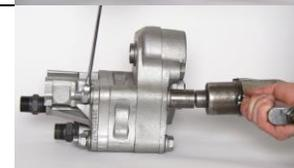
104. Remove the four Lock Nuts (29) and the four Bolts (16) along with eight Lock Washers (15) and eight Flat Washers (16) Examine the bolts and nuts and washers for wear or damage and replace if necessary
