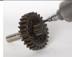
122. Remove the Reduction Gear (20) from the Pinion (20). Examine the gear for chipping of the teeth or spalling of the gear surfaces. Check the shaft for wear or corrosion. Replace if necessary.
