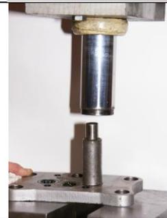
124. Use the fifty ton hydraulic press (on low pressure) to push two new Bearings (27) into the Air Motor Cover (10).
