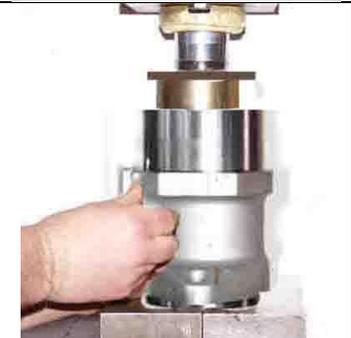
81. When a Chuck Gear (49) is returned to the drill shop with a worn Chuck Bushing (50) the chuck bushing should be removed using the fifty ton hydraulic press in the shop. Examine the Chuck Gear for wear and if it is still in satisfactory condition press in a new Chuck Bushing (50) using the fifty ton shop press. The repaired assembly can be used to replace a worn or damage assembly at the underground drill site.
