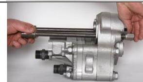
103. Begin disassembly of the failed SASTANMO using a pneumatic impact gun and socket on the head of the Bolt (16) and holding Lock Nut (29) with an open end wrench.
