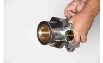
80. Remove the bronze Front Cylinder Liner (30) from the Front Cylinder (31). This is usually done in the drill shop using the fifty ton press. Replace with a new bronze liner using the same shop press to drive it securely into place in the Front Cylinder. This assembly is done in the shop however the assembly could be carried underground to replace at the drill site.
