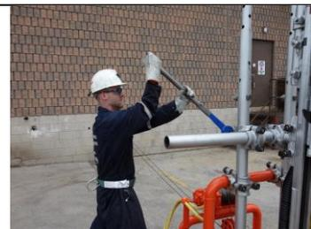
The operator should be sure that the nuts on the universal clamp holding the drill set-up to the sled are tight, so that they do not unscrew while drilling. These nuts must be tight or the drill set-up could rotate on the upper cross bar of the mounting bracket of the sled when drilling is finished and the operator begins loosening other nuts to prepare to move the set-up once again.
