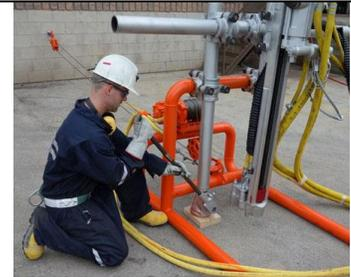
There is no need to tighten the nuts that were loosened to drop the column bars as the drill set-up is not resting securely on the two column bars. All other nuts on the drill set-up should now be tightened to be sure that the entire setup is very rigid.
