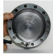
210. Coat the heads of the pistons with grease for lubrication. Place the open end of the two Cylinders (2) over the heads of the protruding Pistons (4) on each side of the head of the Support (18). Drive the Cylinders on using the five-pound plastic mallet.
