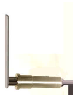
C1512 CHUCK NUT 100% WORN
