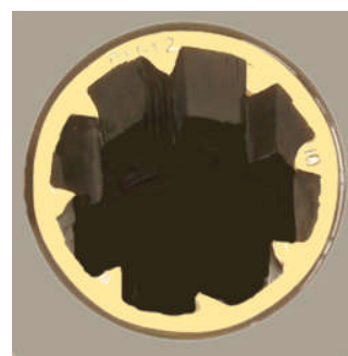
C1512 CHUCK NUT 100% WORN
