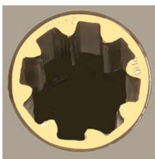
C1512 CHUCK NUT 50% WORN
